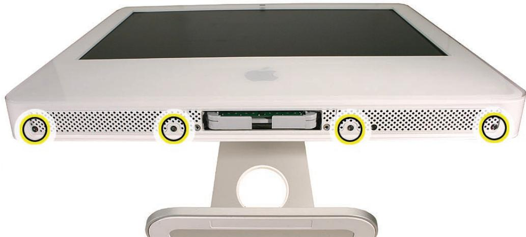
3. Locate the access card. Bending the upper quarter of the access tool card will help engage the latch. **Note:** Refer to [Access Tool Modification](#) in the General Information chapter if the bezel is difficult to open.
