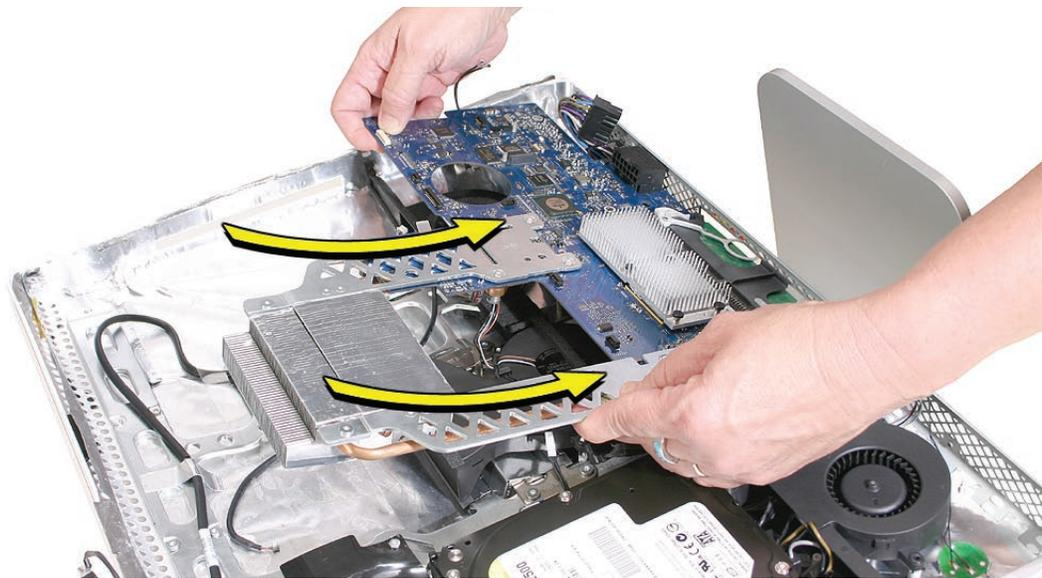
4. At the top of the heatsink, replace the two T6 screws attaching the logic board support bracket to the chassis. **Note:** The L-shaped support brackets must be transferred to the replacement logic board.
