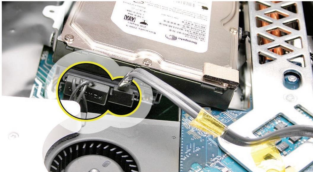
5. If you are replacing the hard drive, transfer the temperature sensor, mounting pins, and the metal mounting bracket to the replacement drive.
