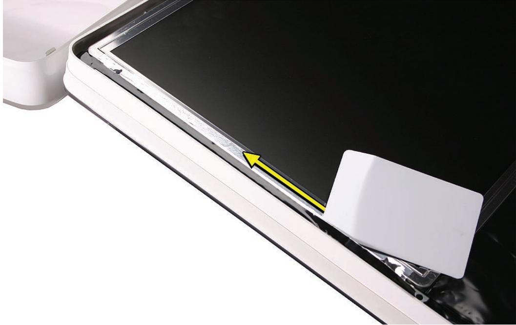
2. Using the access tool or black stick, peel back the black EMI tape stuck along the entire length of the top panel.
