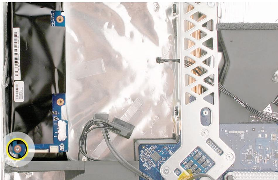
3. Replace the hard drive. Connect the two hard drive cables.
