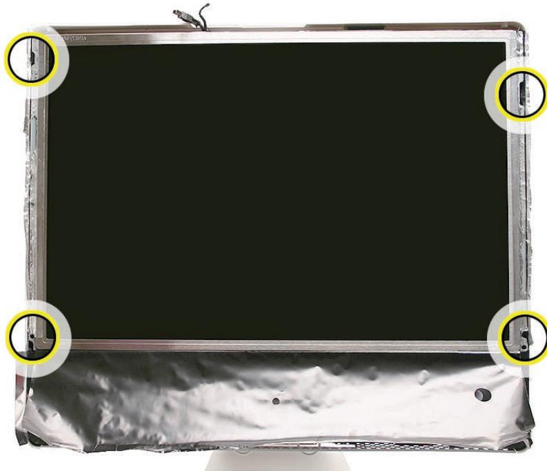
5. Lift the panel up just enough to see the inverter cables on the left side.
