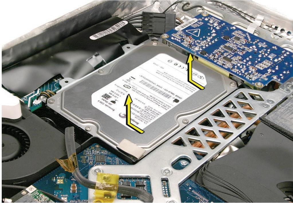
4. Disconnect the hard drive power and data cables from the end of the hard drive.
