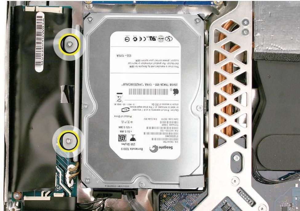
2. Disconnect the hard drive sensor cable from the connector on the logic board. Note the location of the sensor on the side of the hard drive and the routing of the sensor cable under the heat pipes.
